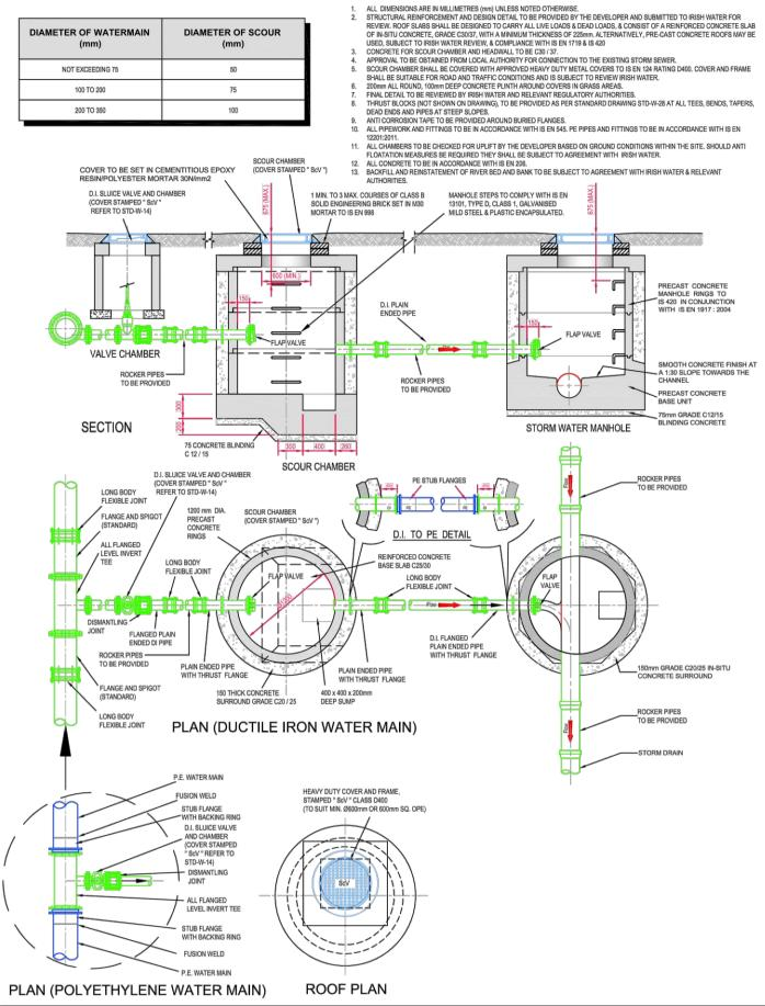
STD-W-30B SCOUR CHAMBER TO STORM SEWER ARRANGEMENTS
